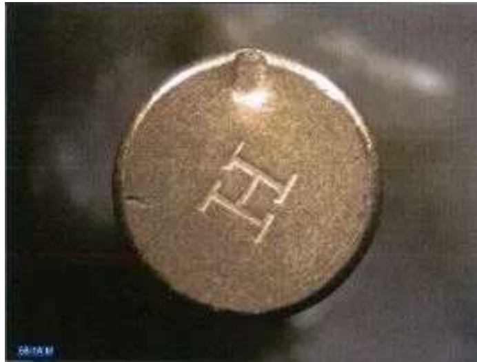
A cartridge case found in the Mele file was shown to the ballistics experts interviewed. The ejector "scratch" is at 9 o'clock. It is visible to the naked eye.
