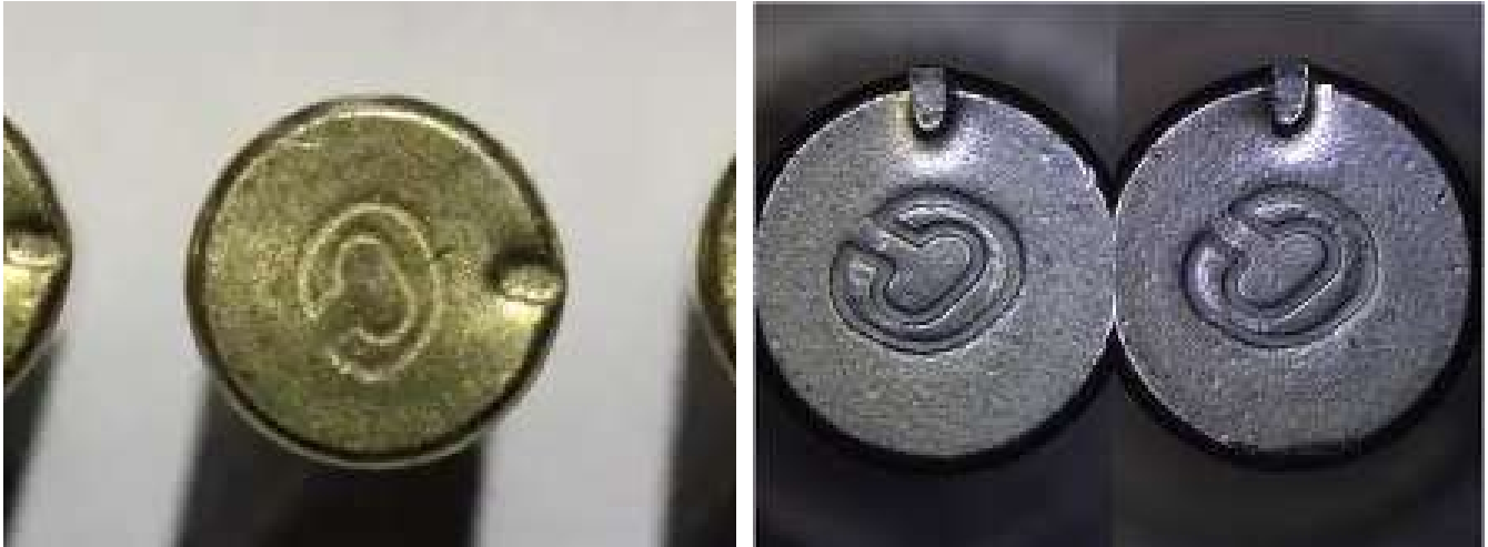
On the left, ejected shell casings from a Beretta 76. On the right, from a rifle. Both are "bar-shaped." Photos taken from my 2021 report, which will be included in the Bevilacqua case file.
