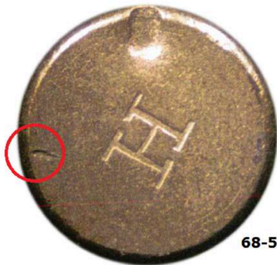
Case in the Mele file. Circled in red, the ejector "scratch" is evident at 9 o'clock.
