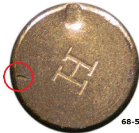
Case in the Mele file. Circled in red, the ejector "scratch" evident at 9 o'clock
