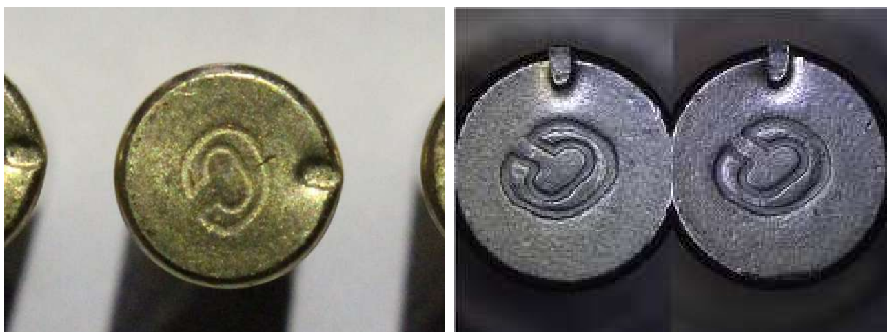
On the left, ejected shells from a Beretta 76. On the right, from a rifle. Both "bar-shaped". Photos taken from a 2021 report of mine that will be included in the Bevilacqua case file
